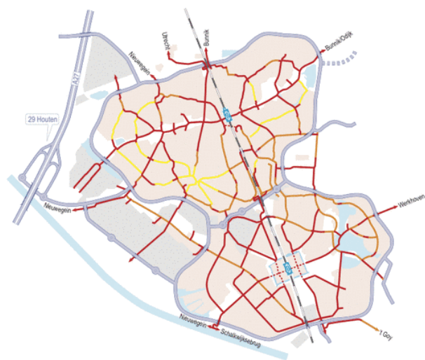
Figure 3-13: Networks in Houten (Gemeente Houten, 2011). The inter-neighborhood connections (red, yellow and orange) are only accessible for non-motorised modes
